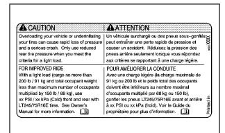
An example of the Improved Ride label is shown here. This label is attached to the lower section of the driver's door edge, for 2500 Series vehicles only.
